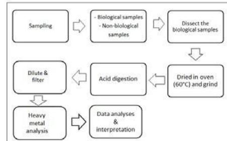
Figure 1: Flow chart of the methodology of this study.
