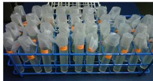
Figure 3.4: Digested samples for the determination of heavy metals by using ICP-MS.
