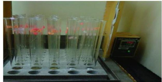
Figure 3.3: Samples digestion by using digestion block.
