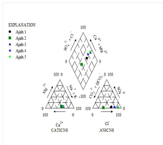
Figure 5: Piper diagram for sample taken from Ajah axis
